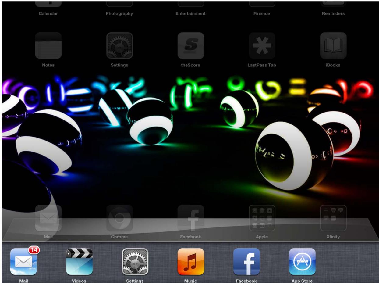
To connect to the projector, double press the home button and slide the active apps bar to the left (by swiping right) until you see the following controls at the bottom of the screen
